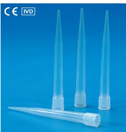
**CAPACIDAD 1000-5000 µL****Compatibilidad:** Kartell®, Gilson®, Socorex®, Nichiryo®**CAPACITY 1000-5000 µL****Compatibility:** Kartell®, Gilson®, Socorex®, Nichiryo®**CAPACIDADE 1000-5000 µL****Compatibilidade:** Kartell®, Gilson®, Socorex®, Nichiryo®
